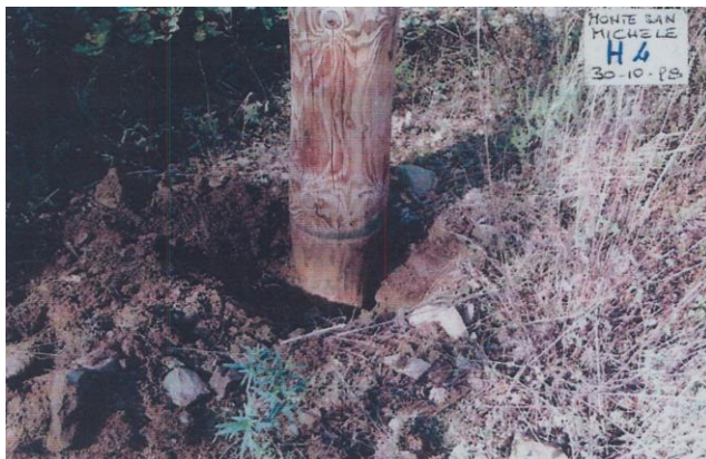
Pole impregnated with Tanalith – E after 6 years (Italy)
