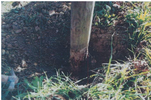
Unimpregnated pole after 4 years, visible damage (Italy)
